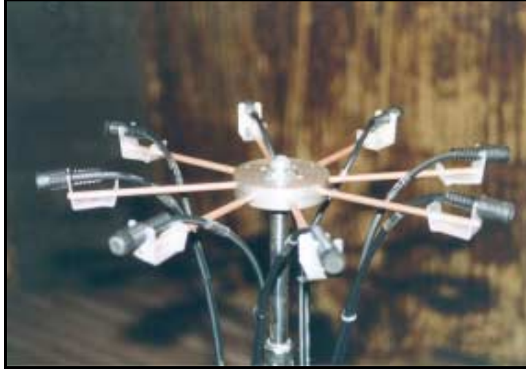
Fig. 2. The microphone matrix used for sound acquisition
